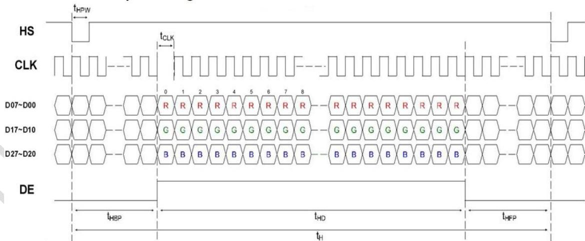
Figure 5.2.1 Horizontal input timing
