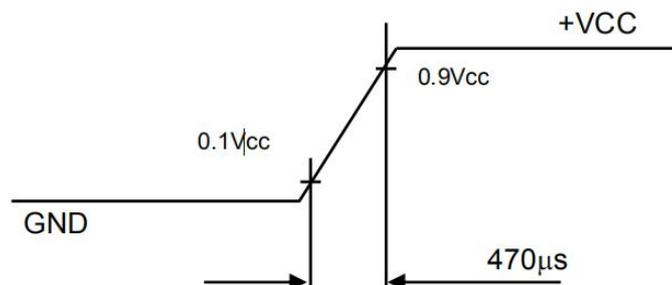
Figure 4.2 Inrush current test condition
